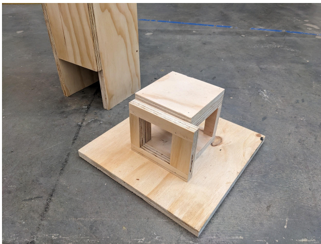
Figure 4. This “house” as I came to call it was nailed to the “foot” (large square) with a facing piece matching the space cut from the bottom of the leg. The opening is 3” x 3” to accept the 3” x 3” beam that connects the legs. These had a tight friction fit to the legs, but did not stop the legs from pivoting when forces were applied perpendicular to the open face.
