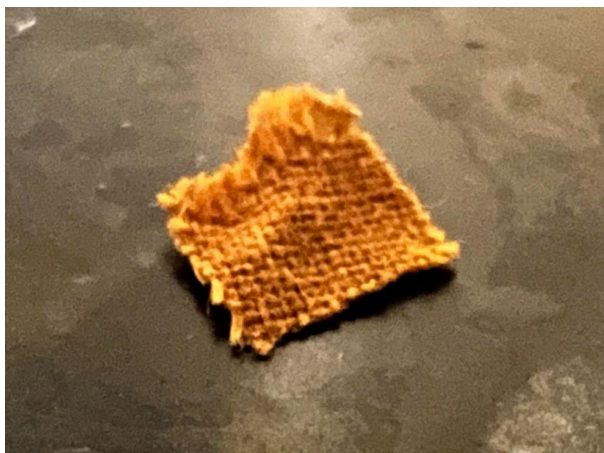
Figure 22. 0.5 cm x 0.5 cm swatch of silver-enabled fabric used for the release study
