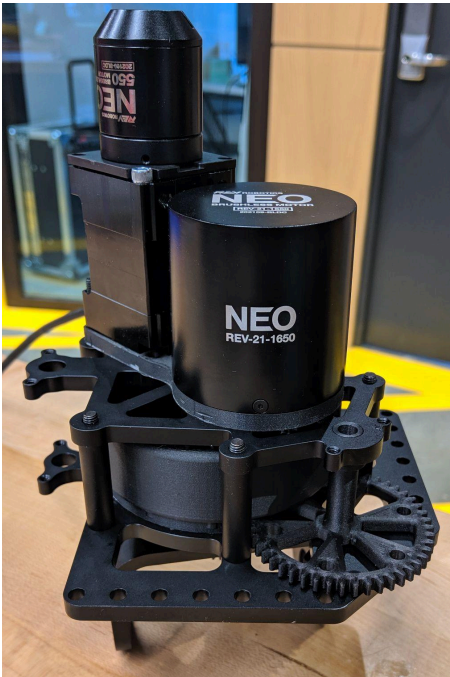
Figure 3. Motors attached to housing frame
