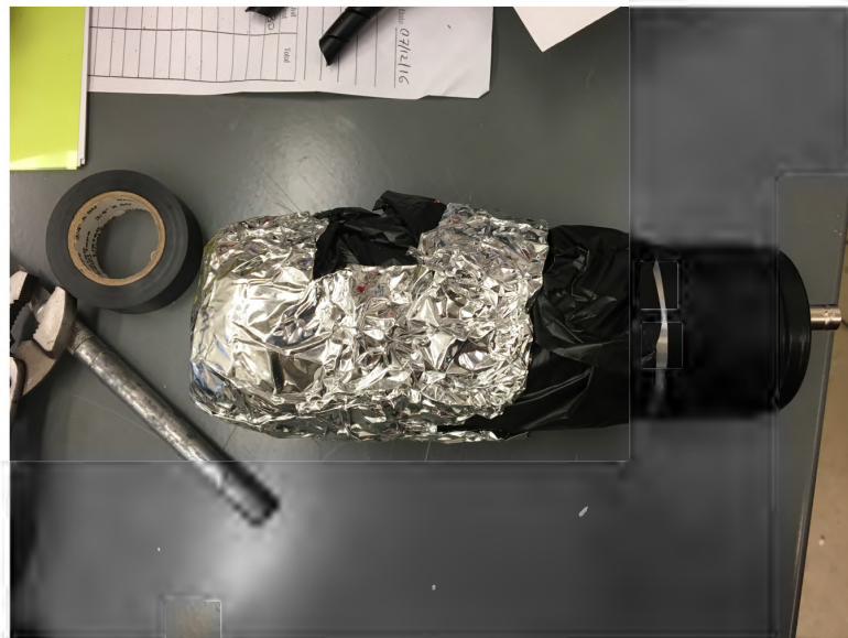
Figure 5.10: A photograph of the plastic scintillator coupled to a PMT, though most of the detector is hidden by the case and the foil.
