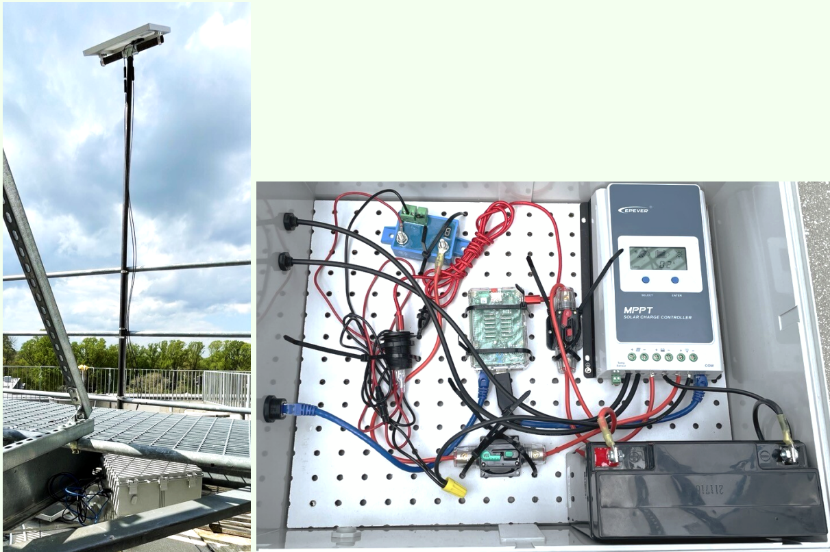
Figure 4. Left: Photo of the Swarthmore Solar Protocol server on the back rack of the Singer Hall Solar Lab, with the solar panel mounted on an adjustable mount designed by J Jaoudi and the enclosure on an acrylic shelf below the rack also designed by Jaoudi. Right: A photo of the inside of the enclosure, notably the Raspberry Pi is located in the center mounted with zip-ties to a perforated board. Next to it on the right are the MPPT charge controller and battery.
