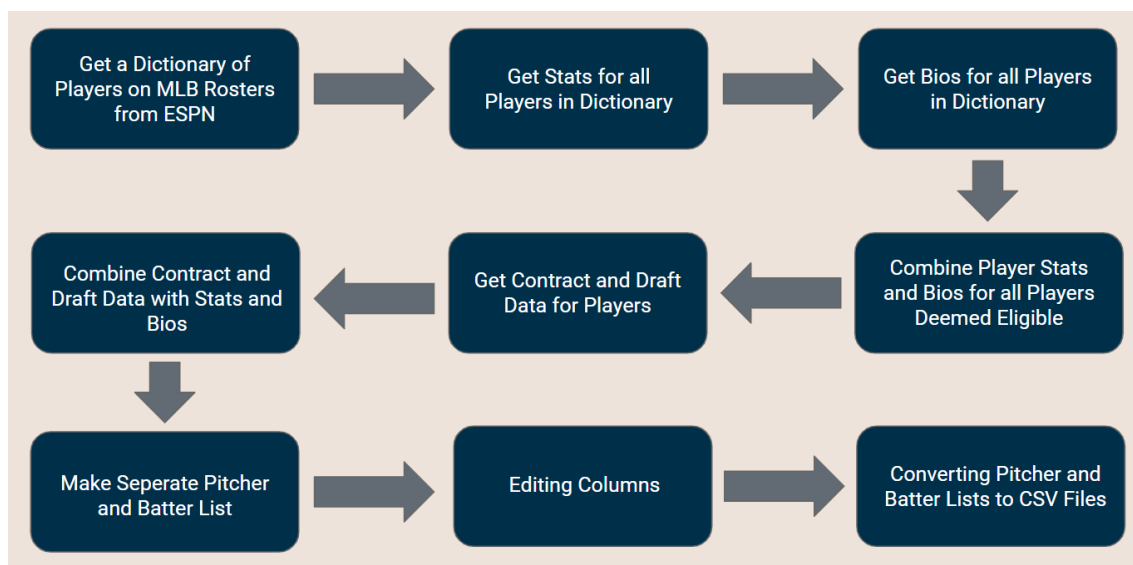
Figure 1: Overview of the Structure of the Code Used to Create Datasets
