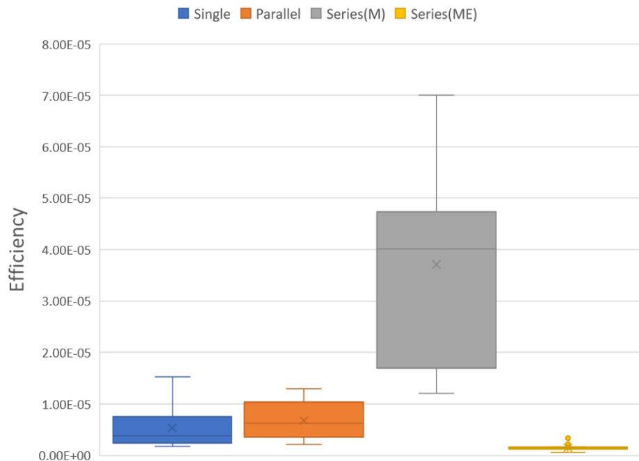
Fig. 8. Box-and-whisker plot of the efficiencies of the four different types of twisted-and-coiled actuator systems. (M) means only mechanically in series, but electrically in parallel, while (ME) means both mechanically and electrically in series. The vertical axis of this plot is in log scale.
