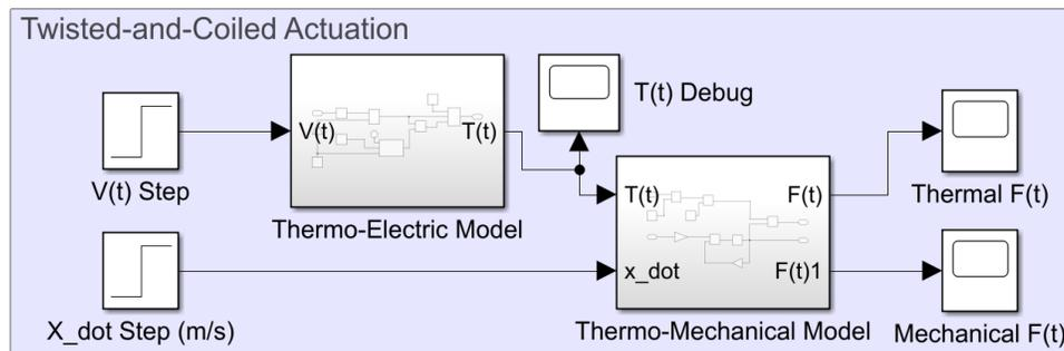
Fig. 4. The mathematical model of a twisted-and-coiled actuator
