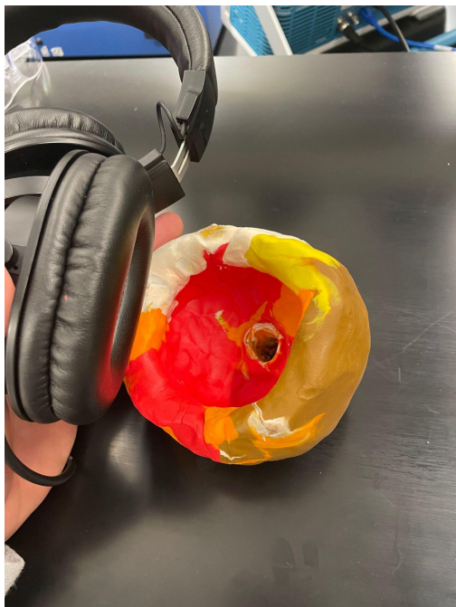
Figure 8 - A molded “ear” used in testing
