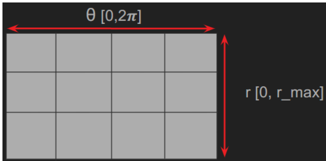
Figure 6: Visualization of the Hough space for line detection
