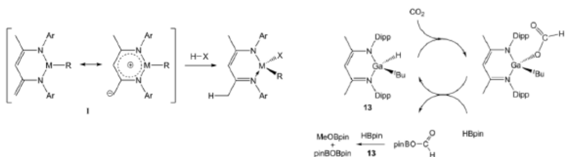
Scheme 2. H–X bond activation by a β-diketiminato gallium complex, followed by selective reduction of CO 2 by a β-diketiminato gallium hydride complex to form a methanol derivative. Reproduced from Abdalla et al. 2015. 27
