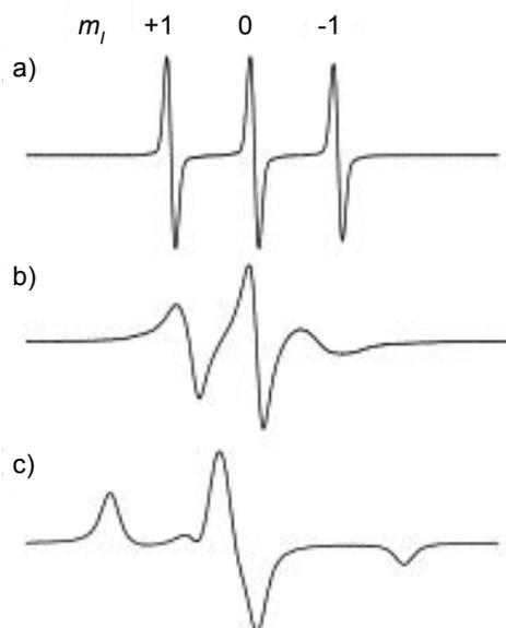
**Figure 2.9. The CW EPR spectra of MTSL (a) in solution, (b) bound to residue on  $\alpha$ -helix protein, (c) in frozen solution.** Adapted from Klug et al., 2008.<sup>36</sup>
