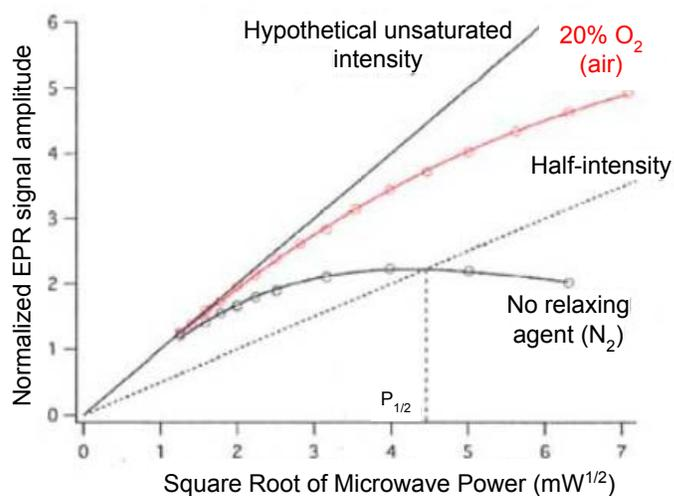
**Figure 2.10. Representative oxygen accessibility from power saturation studies.** EPR intensity has a linear relationship with the square root of microwave power (black straight line). Half intensity is shown with a dotted line. The EPR signal trend of various microwave powers in the presence of a non-paramagnetic reagent ( $N_2$ ) is shown with the black curve line and in the presence of a paramagnetic reagent ( $O_2$ ) is shown with the red curve line.
