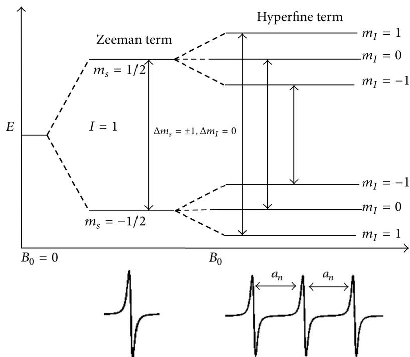
**Figure 2.7. Energy level diagram of a free spin-label in solution in the presence of a magnetic field  $B_0$ .** The energy splitting of an electron due to Zeeman splitting and Hyperfine splitting are shown on the top. EPR spectra in the absence and presence of a  $^{14}\text{N}$  nucleus with  $I = 1$  hyperfine interaction is shown in the bottom. Taken from Sahu et al., 2018.<sup>35</sup>
