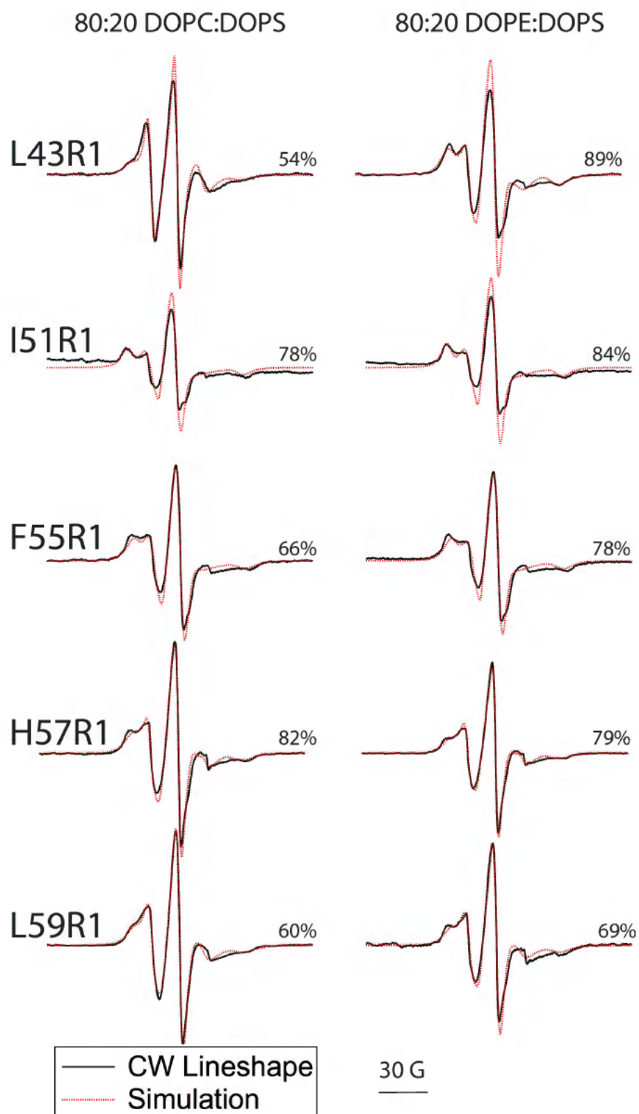
Figure 4.3.3. Spectral simulations (red) of dilute labelled CW EPR spectra (black) for five selected labelling sites in cubic (PE) and lamellar phase (PC) lipid environments. Percent of immobile component population is listed to the right.
