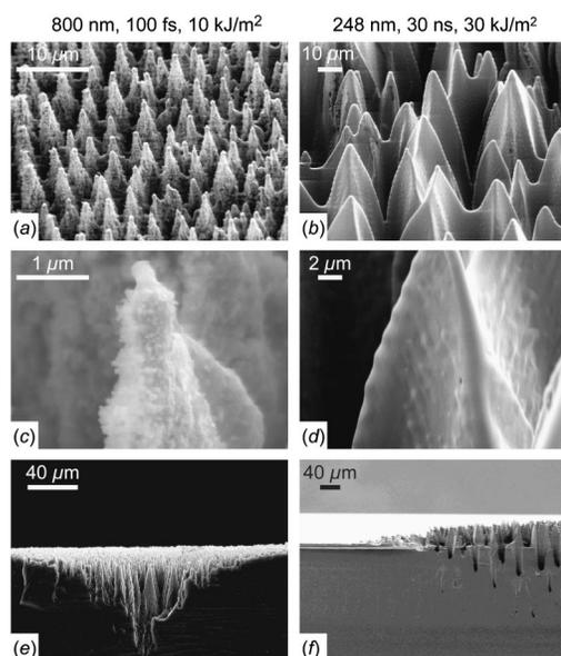
FIG. 1. Scanning electron micrographs of laser-microstructured Si surface formed in SF<sub>6</sub> [(a), (c), (e)] with fs laser pulses, and [(b), (d), (f)] with ns laser pulses. In (a)–(d) the sample is viewed at 45° to the normal; in (e) and (f) the sample is snapped in half and viewed edge-on.
