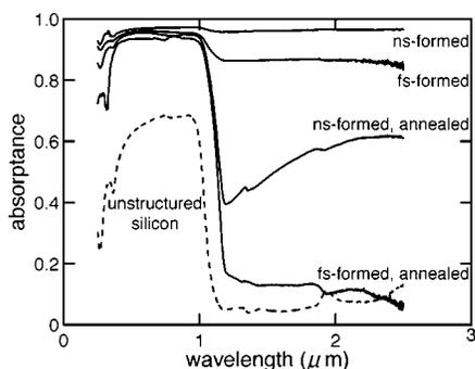
FIG. 2. Dependence of absorbance ( $A$ ) on wavelength of fs-laser-formed and ns-laser-formed microstructures, before and after thermal annealing at 875 K for 45 min in flowing Ar. The absorbance of the unstructured Si substrate is also shown.
