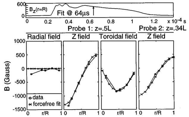
FIG. 7. Force free equilibrium data in the large flux conserver. Early in decay (64  $\mu\text{s}$ ) with flux function as depicted in Figure 5(a).
