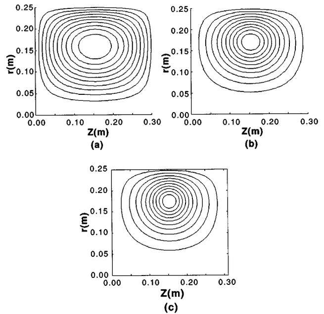
FIG. 5. Zero pressure solutions for the poloidal flux with various  $\lambda$  profiles. (a) Constant  $\lambda$  appropriate for early in decay, (b) linear  $\lambda(\Psi)$  and (c) quadratic  $\lambda(\Psi)$  with  $\bar{\lambda}=29 \text{ m}^{-1}$ ,  $\alpha \approx 0.22$ , and  $\gamma \approx 0.75$  appropriate for late in decay.
