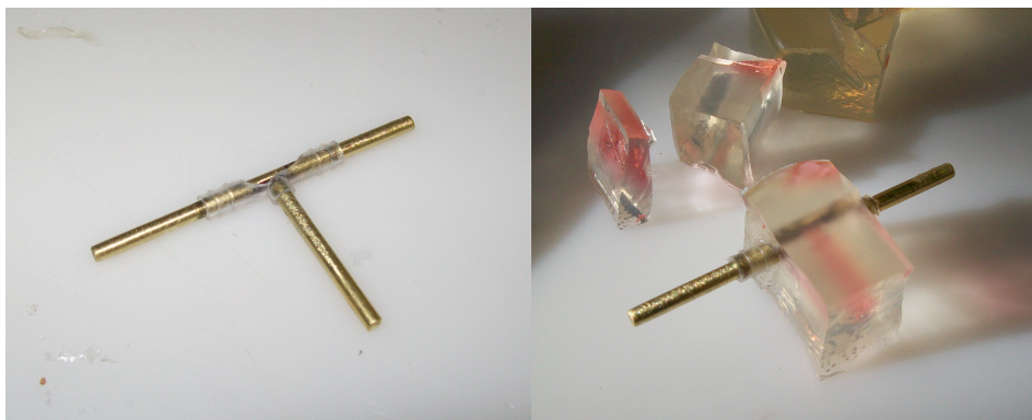
FIGURE 1A AND 1B. Fabrication of sample holders shown, in which 10% gelatin surrounds a T-shaped channel. The top part of the “T” is formed via a straight length of tubing with a brass rod inserted through it (shown). The descending leg of the “T” is formed by another brass rod. Following gel setting in a mold, the brass rods are removed and the sample is formed in the leg (shown as pink).
