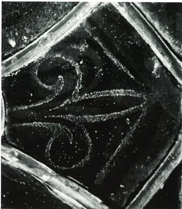
FIG. 7. Details of Fig. 4: exterior views with surface light, highlighting corrosive deposits; interior painting is visible through the transparency of the glass. (Photos: author)
