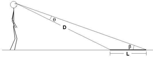
Figure 1. Exocentric in-depth distance,  $L$ , can be estimated using the visual angle subtended,  $\theta$ , the viewing distance,  $D$ , and the optical slant,  $\beta$ . That is, according to the law of Sines,  $(\sin \theta)/L = (\sin \beta)/D$ . Thus,  $L = D \sin \theta / \sin \beta$ . Overestimation in perceived  $\beta$  would result in underestimation in perceived  $L$ .
