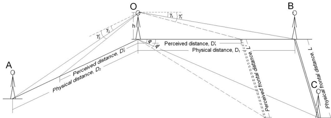
Figure 13. Diagram illustrating the geometry of the spatial variables in the experimental setup used in Experiment 2. Note that all the experimenters were on a level ground plane.
