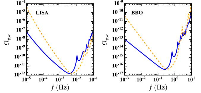
FIG. 5. Left panel: The sensitivity curve for  $\Omega_{\text{gw}}^{(I,V)}$  for LISA assuming a separation between the two observatories of  $D/L = 7$ , and a 10-year-long observation. The solid blue curve shows the sensitivity to the intensity and the dashed orange curve shows the sensitivity to the circularly polarized background. Note that the sensitivity curve for  $V$  has a smaller opening angle. Right panel: The same as in the left panel but for BBO and  $D/L = 2$ .
