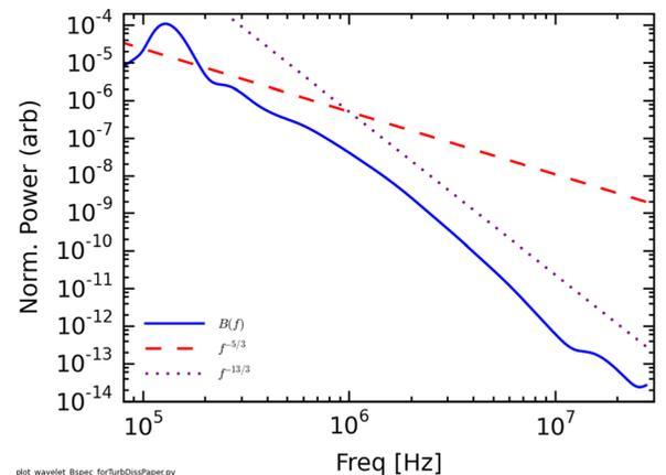
FIG. 2. Fluctuation magnetic field spectrum on logarithmic axes consisting of the sum of  $B_r$ ,  $B_\theta$ , and  $B_z$ , summed over fifty shots. The dashed orange line indicates Kolmogorov scaling ( $f^{-5/3}$ ), while the dotted purple line indicates steeper scaling ( $f^{-13/3}$ ).
