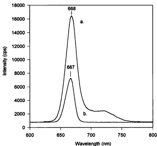
FIGURE 2 Emission spectra of 6.0  $\mu\text{M}$  chlorophyll *a* in acetone. Temperature: 25°C. Spectral bandpass: 1.9 nm. (a) fluorescence spectrum excited at 430 nm; (b) synchronous emission spectrum, with an interval of 0.0 nm between the excitation and emission wavelengths. The spectra are plotted on the same intensity scale to show that the synchronous emission signal is generally less intense than the fluorescence signal.
