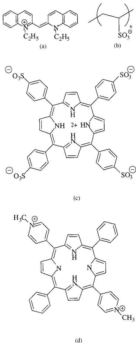
FIGURE 1 Structures of the reactants. (a) Pseudoisocyanine ( $\text{PIC}^+$ ). (b) Polyvinylsulfonate (PVS). (c) The diacid form of tetrakis-4-sulfonatophenylporphyrin ( $\text{H}_4\text{TPPS}_4^{2-}$ ). And, for comparison, (d) the free-base form of *trans*-bis(*N*-methylpyridinium-4-yl)diphenylporphyrin (*trans*- $\text{H}_2\text{Pagg}$ ).
