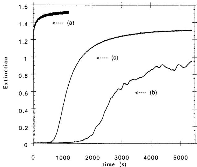
FIGURE 3 Reaction profiles for the aggregation of three  $H_4TPPS_4^{2-}$  solutions differing only in the protocol of mixing. See Materials and Methods for details. (a) Mixing method I. (b) Mixing method II, no stirring. (c) Mixing method II with stirring.
