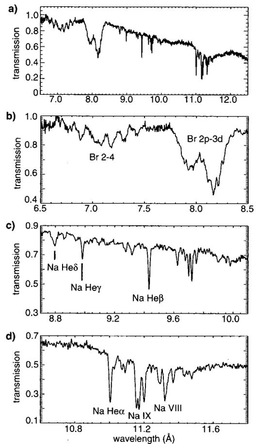
FIG. 7. Transmission measured as a function of wavelength for a radiation-heated CH-tamped NaBr sample. The entire spectrum is shown in (a) and blowups of the Br absorption lines, the Na high- $n$  transitions, and the Na 1–2 transitions are shown in (b), (c), and (d), respectively.
