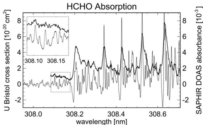
**Fig. 1** Comparison of the absorption spectrum of Pope *et al.* (2005) (thick line, left axis) and the HR DOAS absorbance measured in the SAPHIR chamber (thin line, right axis; see text for details). The inset denotes the spectral range where HCHO lines strongly overlap with the OH  $Q_1(3)$ ,  $Q_{21}(3)$ , and  $P_1(1)$  lines.
