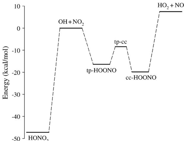
**Fig. 4** Energetics of the OH + NO<sub>2</sub> system, showing the relative energies of nitric acid (HONO<sub>2</sub>), the *cis-cis* (*cc*) conformer of HOONO and the *trans-perp* (*tp*) conformer of HOONO. The energy of the *trans-perp/cis-cis* isomerization barrier (*tp-cc*) is also shown.
