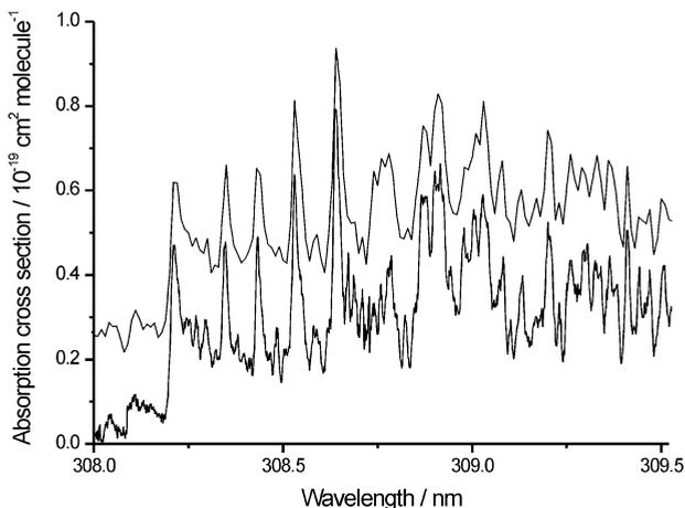
**Fig. 2** Absorption spectra of formaldehyde in the air wavelength region 308–309.5 nm obtained at resolutions of 0.01 nm (grey line, offset vertically by  $0.2 \times 10^{-19} \text{ cm}^2 \text{ molecule}^{-1}$  for clarity) and  $<0.0016 \text{ nm}$  (black line).
