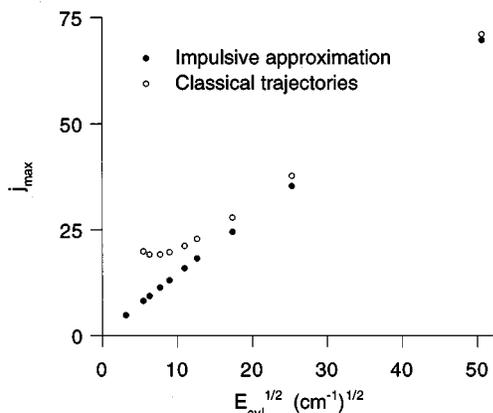
FIG. 12. Calculated variation of  $j_{\max}$  on  $E_{\text{avl}}^{1/2}$  for two classical models for the dissociation of NeBr<sub>2</sub>. The angular momentum,  $j_{\max}$ , is plotted in units of  $\hbar$ .
