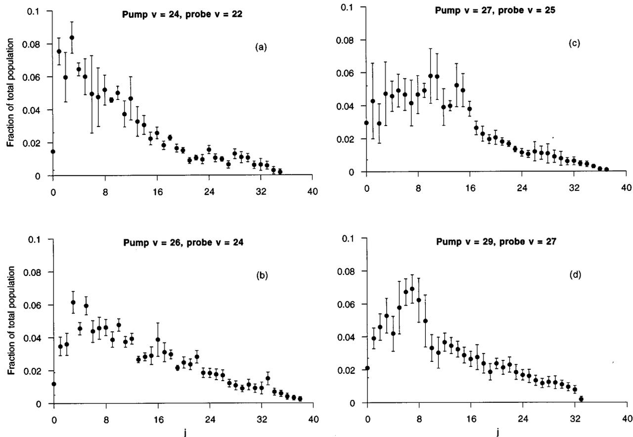
FIG. 5. Distributions of rotational states resulting from  $\Delta v = -2$  dissociation events in NeBr<sub>2</sub>. Each distribution is normalized such that the sum of the populations equals one. (a)  $v = 24 \rightarrow v = 22$ ; (b)  $v = 26 \rightarrow v = 24$ ; (c)  $v = 27 \rightarrow v = 25$ ; (d)  $v = 29 \rightarrow v = 27$ .
