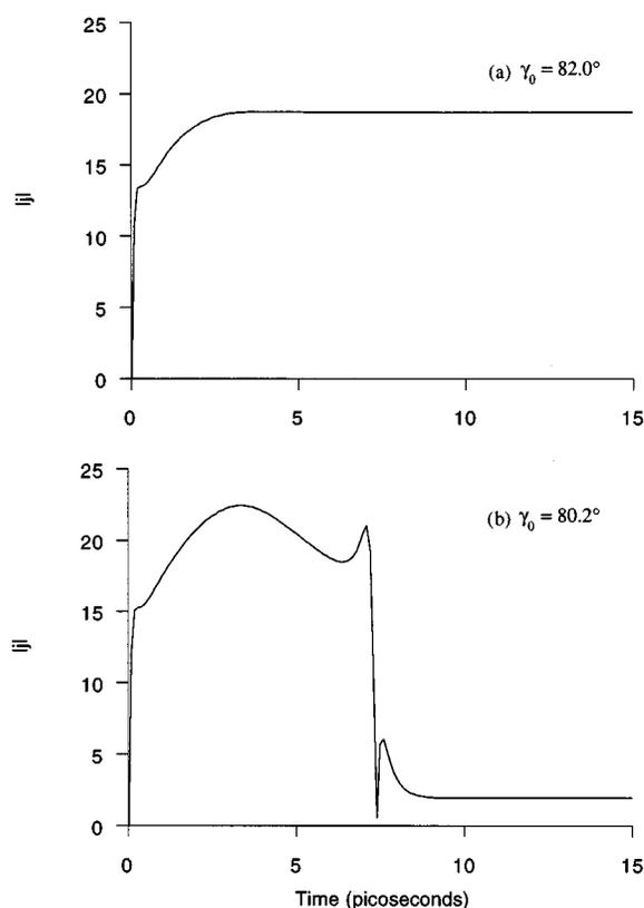
FIG. 10. Temporal evolution of the angular momentum for two of initial conditions displayed in Fig. 9. The magnitude of the angular momentum,  $|j|$ , is plotted in units of  $\hbar$ . (a)  $\gamma_0=82.0^\circ$ ; (b)  $\gamma_0=80.2^\circ$ .
