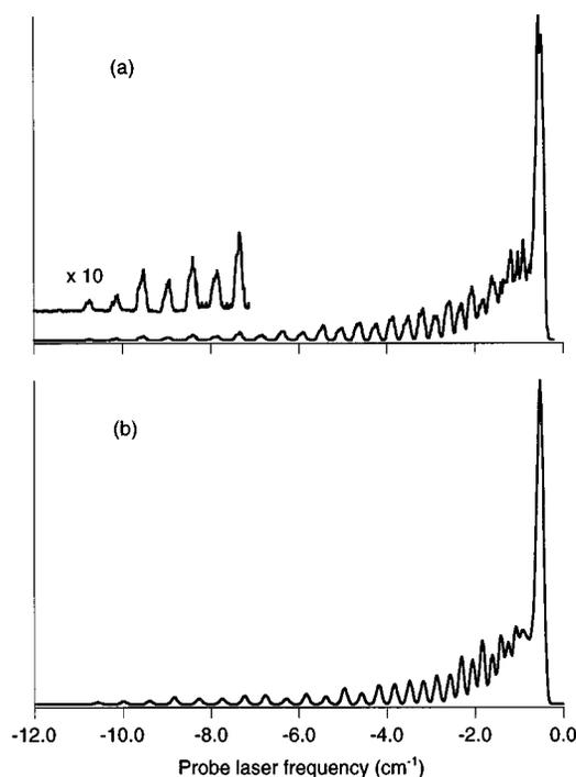
FIG. 1. (1,14)  $E \leftarrow B$  fluorescence excitation scan of Br<sub>2</sub> fragments from the dissociation of NeBr<sub>2</sub> prepared in the  $v=15$  level of the  $B$  electronic state. (a) Experimental data; (b) simulated spectrum using rotational state populations derived from a least-squares fit to the experimental data.
