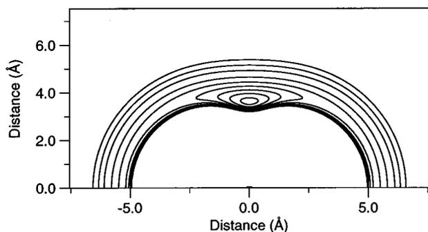
FIG. 6. Model potential energy surface for NeBr<sub>2</sub>. The origin of the coordinate system is fixed at the center of mass of Br<sub>2</sub>. The energy contours are drawn at 10 cm<sup>-1</sup> intervals, with the outermost contour lying -10 cm<sup>-1</sup> relative to the energy of separated Ne+Br<sub>2</sub>.
